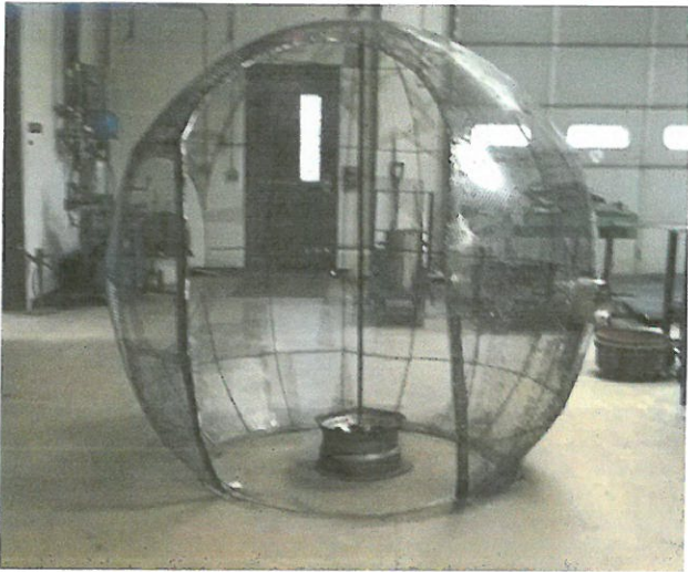
Entry door cut and reinforced
